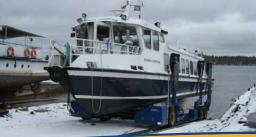
SUBLIFT is made for easy and safe dry docking and launching of sailing and motor boats on ramps and slipways. Typical usage is docking for fast service, cleaning of hulls and for winter season storage.
