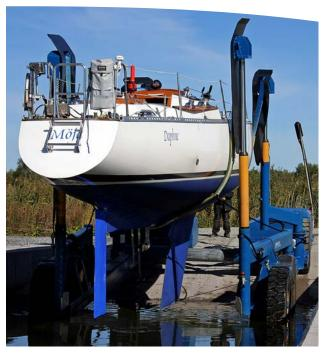
**The SUBLIFT 25t** is a workhorse used by both marinas as well as by boat clubs. It is equipped with slings on two pairs of hydraulic lifting arms that can rotate either manually or with optional hydraulic cylinders to fit boat widths up to 4.9 meters. The hoist is designed for up to 25 ton boats.
