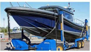
**The SUBLIFT 12t** is the smallest and the most popular model in the range. Typical users are marinas and boat clubs. It is equipped with slings on two pairs of hydraulic lifting arms that can rotate manually to fit boat widths up to 4.8 meters. Maximum boat weight is 12 ton.
