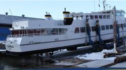
The SUBLIFT 90t is a heavy duty machine for the marina that handles larger vessels. It is equipped with three pairs of hydraulic lifting arms with double slings.
