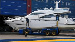
The SUBLIFT 25t is a workhorse used by marinas and boat clubs with a wide range of boats. It is equipped with slings on two pairs of hydraulic lifting arms.
