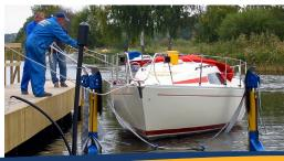
The SUBLIFT 12t is used by marinas and boat clubs. It is equipped with slings on two pairs of hydraulic lifting arms. Maximum boat weight is 12 ton.
