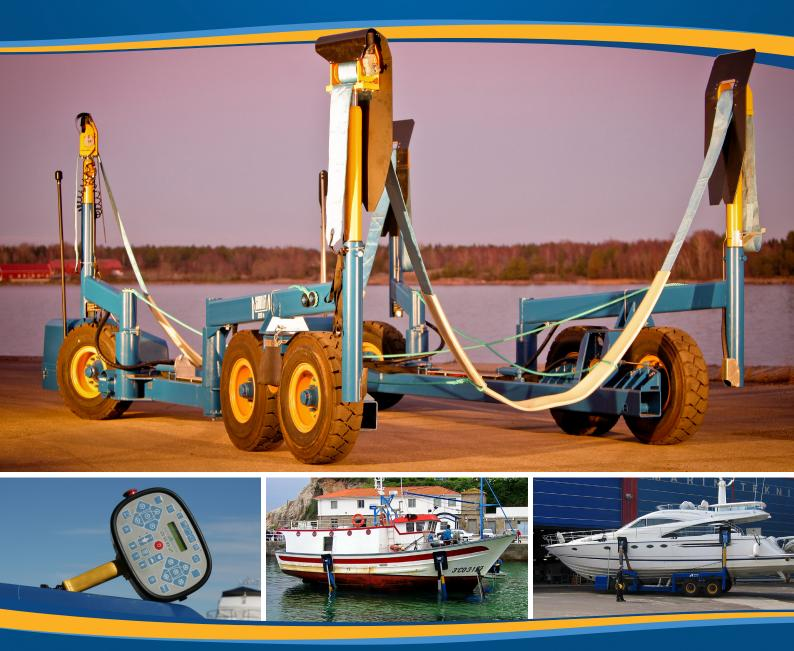
The SUBLIFT 25t is a workhorse used by marinas and boat clubs with a wide range of boats. It is equipped with slings on two pairs of hydraulic lifting arms. The hoist is designed for up to 25 ton boats.
