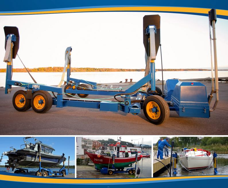
The SUBLIFT 12t is used by marinas and boat clubs. It is equipped with slings on two pairs of hydraulic lifting arms. Maximum boat weight is 12 ton.
