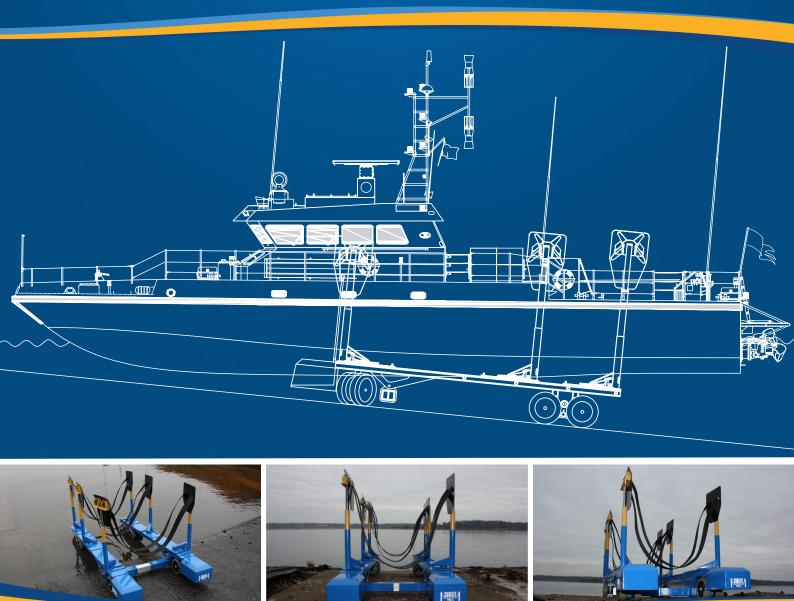
The SUBLIFT 75t is under development based on the experiences made on the 65 and 90 ton models. It is the choice for the yard that service a larger range of boats. It is equipped with double slings on three pairs of hydraulically controlled lifting arms making the hoist most the flexible. The full capacity is 75 ton.
