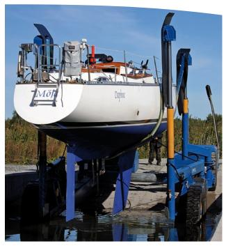
**The SUBLIFT 25t** is a workhorse used by both marinas as well as by boat clubs. It is equipped with slings on two pairs of hydraulic lifting arms that can rotate with hydraulic actuators to fit boat widths up to 4.9 meters. The carriage is designed for up to 25 ton boats.
