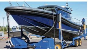
**The SUBLIFT 12t** is the smallest and the most popular model in the range. Typical users are marinas and boat clubs. It is equipped with slings on two pairs of hydraulic lifting arms that can rotate manually to fit boat widths up to 4.2 meters. Maximum boat weight is 12 ton.
