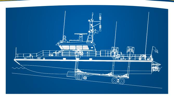
The SUBLIFT 75t is under development based on the experiences made on the 65 and 90 ton models. It is the choice for the yard that service a larger range of boats. It is equipped with double slings on three pairs of hydraulically controlled lifting arms that can move axially and rotate to fit boat widths up to 7.6 meters. With all lifting arms movable this is the most flexible carriage. Using two out of three slings smaller boats can be taken. The full capacity is 75 ton.
