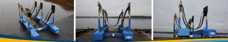
The SUBLIFT 75t is under development based on the experiences made on the 65 and 90 ton models. It is the choice for the yard that service a larger range of boats. It is equipped with double slings on three pairs of hydraulically controlled lifting arms making the carriage most the flexible. The full capacity is 75 ton.
